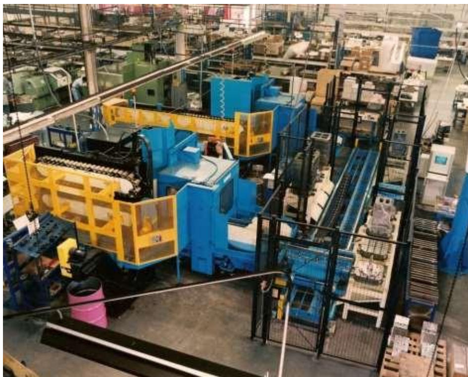
Fig. 68 A five-machine flexible manufacturing system for machining (photo courtesy of Cincinnati Milacron)
